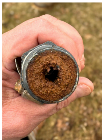
Iron in water is particularly troublesome because pathogenic bacteria like E. Coli thrive on iron deposits in pipes (left). Only mechanical filtration (right multi-stage system) reliably extracts it.
